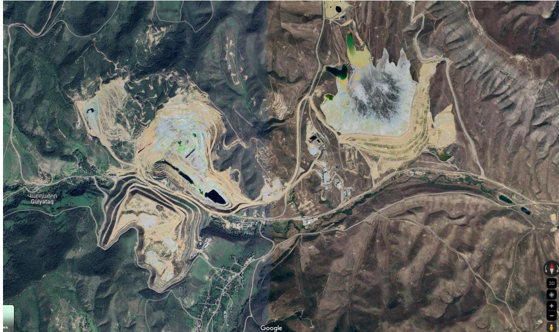
Demirli open pit (to the left), tailings dam (to the right) and the processing facilities plan view
